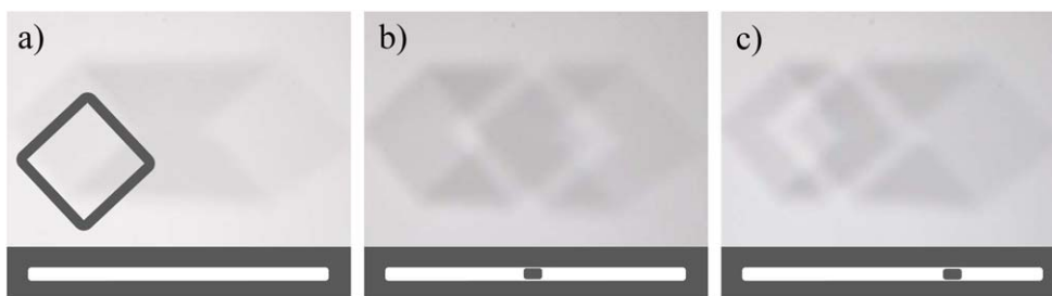
Figure 11. A square frame of paper, suspended by a nylon thread, is illuminated by a horizontal rod lamp (a). If the lamp is covered at one point, a bright shadow appears in the diffuse shadow of the frame (b and c).
